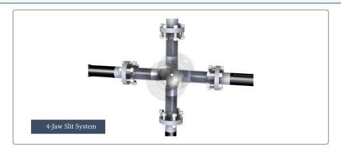
The 4-Jaw Slit System can be used for analyzing as well as forming the size and shape of a charged particle beam. It consists of four plates which can be moved individually from an out-of-beam position into the beam. The position of the slits is adjustable with sub-millimeter precision.
