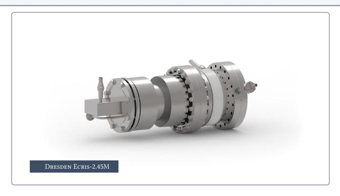
The Dresden ECRIS-2.45M is an electron cyclotron resonance ion source designed to produce low charged single particle and molecular ion beams in the range of several  $100\,\mu\text{A}$ . Because of its compact design and few infrastructural requirements the Dresden ECRIS-2.45M can easily be integrated into existing beamlines or mounted on a high voltage terminal of electrostatic accelerators.
