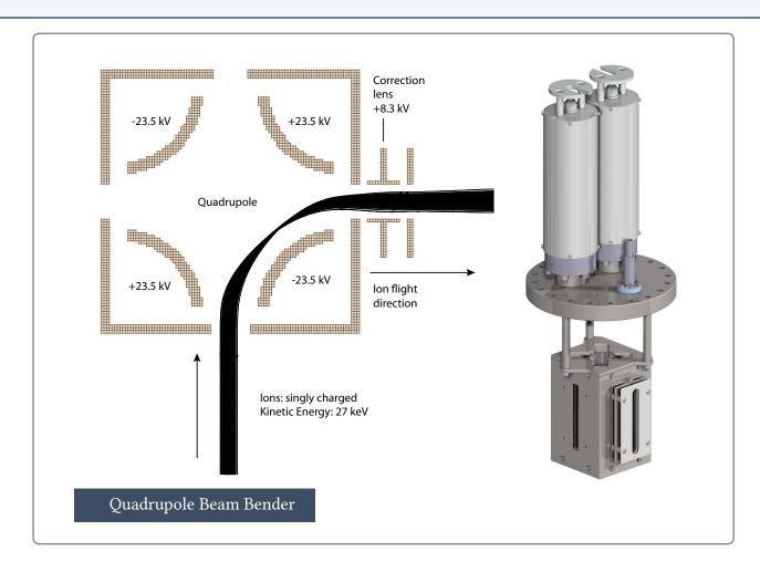
The DREEBIT Quadrupole Beam Bender is an ion optical device designed to bend charged particle beams with kinetic energies of up to  $25\,\mathrm{keV}$  per charge by an angle of 90°. The deflection is realized by quarter-pipe electrodes set up perpendicularly to the direction of the incoming ion beam in a typical electrostatic quadrupole arrangement.
