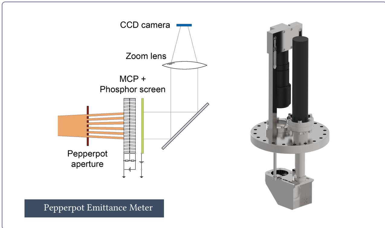
The Pepperpot Emittance Meter is an imaging system which allows for detecting and evaluating beam parameters of particles as well as x-rays in real-time. The setup is mounted onto a single DN 160 CF flange with a linear motion vacuum feedthrough, two SHV high voltage feedthroughs, a glass viewport, and a camera holder. The main components of the diagnostics unit are a pepperpot-like pinhole mask, a micro channel plate (MCP) and a phosphor screen assembly, a mirror, and a CCD camera.
